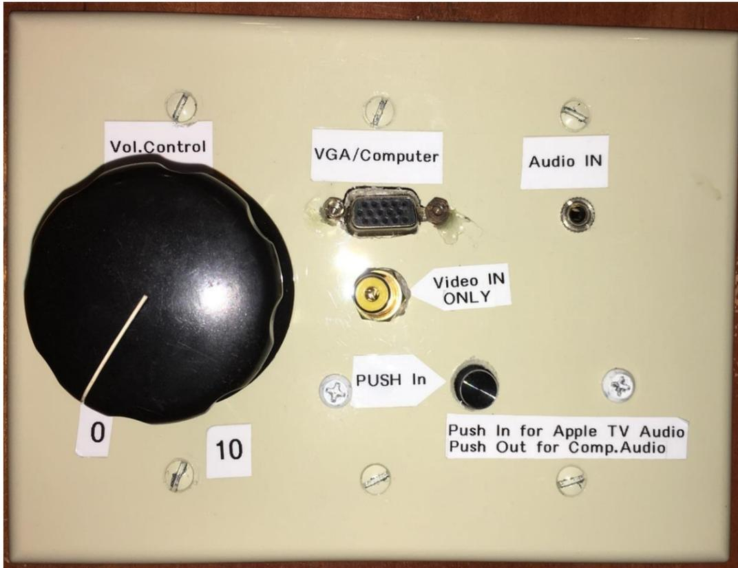
**1.) If you are using audio from your laptop, Iphone, etc.** Then plug in 1/8" jack, one end to your laptops Headphone Jack and make sure your computers volume about half way. Plug the other end of the cable into the wall plate labeled **Audio IN** and turn the Volume Control up half way and make sure the **Comp. Audio button** is in the out position. Then adjust your device's volume or the wall volume control to get the best sound for you.
