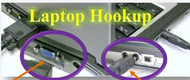
Connect VGA cable from lectern, to the back of your laptop. **NOTE:** If the image does not appear on the screen with the projector ON, you may need to press the FN key + the F8 to activate the video port on your laptop. (Maybe different for some laptops)
